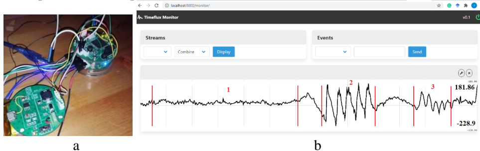
Fig.6. EEG signal measurement process: a – electronics board, b – dry electrodes, 1 – eyes closed, 2 – chewing, 3 - blinking
