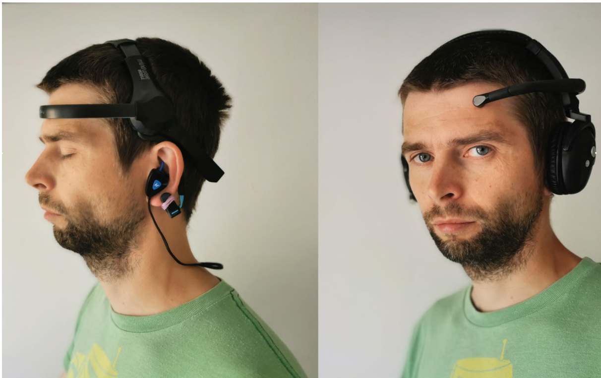
Figure 4.3: Photo of NeuroSky headsets. Mindwave (left) with additional Bluetooth headphones and Mindset (left) with built-in over-ear headphones.
